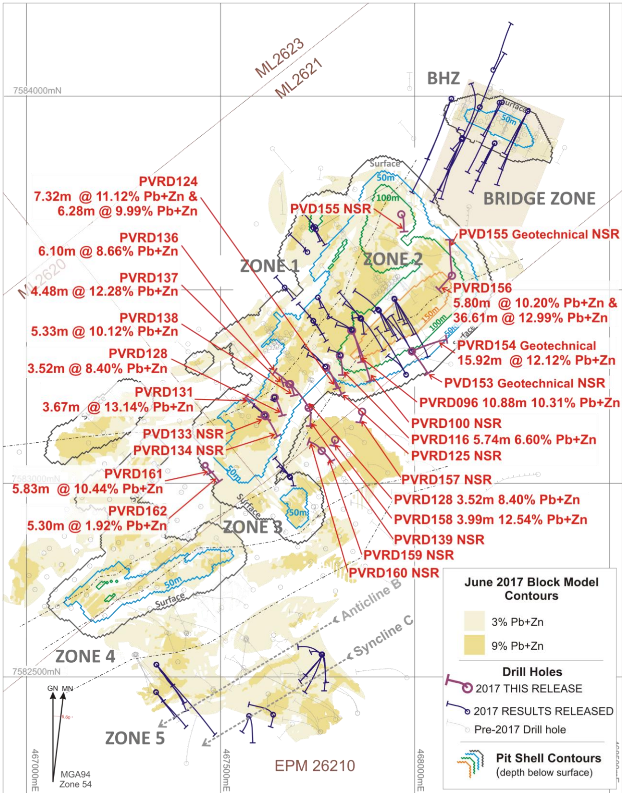
Figure 1. Surface Map Showing 2017 Mineral Resource Block Model Contours, Pit Shell and Location of Current Results and 2017 Completed Holes
