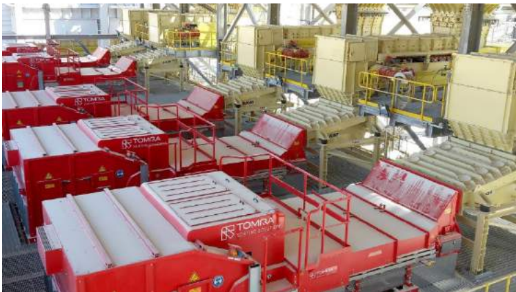
TOMRA COM XRT 2.0 Units at a phosphate mine (source: TOMRA)
